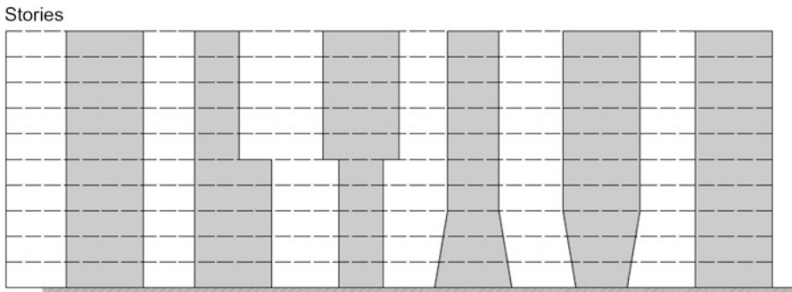
Fig. 21.43 Elevation configuration for shear walls
