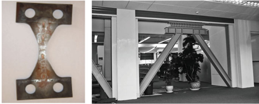
Fig. 17.5 Example of ADAS dampers
